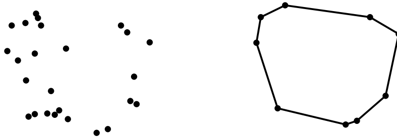
Figure 5. Left: Point cloud, Right: Convex hull in two dimensions
