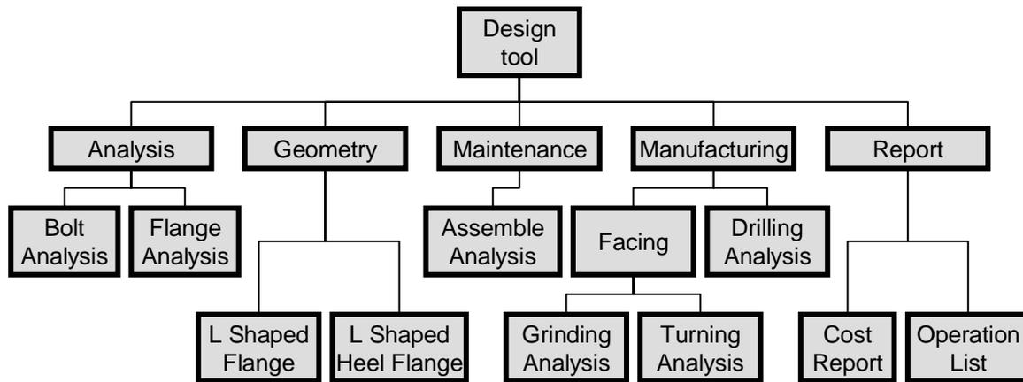
Figure 2. The structure of the multidisciplinary design tool.
