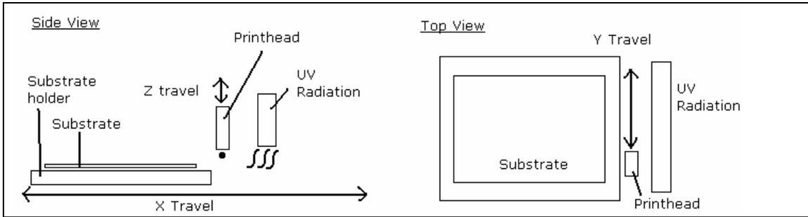
Figure 5: The three axes of motion. As an operator of the machine would see it; the substrate table moves left to right (X axis) passing the substrate under the print-head and the UV radiation. The printhead is able to index, either toward or away from the operator (Y axis), this allows the print-head to cover more of the substrate with more swathes of the image. The distance of the print-head above the substrate is maintained at a safe working distance (Z axis.)
