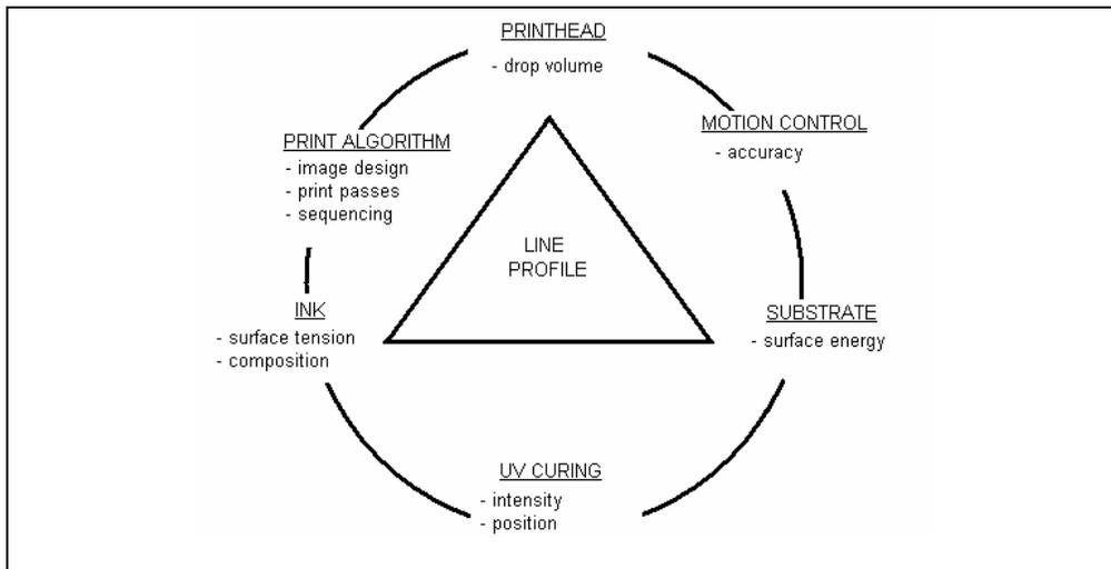
Figure 7: The ink-jet triumvirate expanded to include the secondary subsystems and individualised for line profile.
