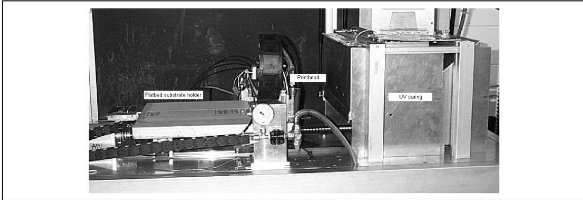
Figure 4: The core parts of the prototype: A substrate held in a substrate holder, which receives the ink as it passes under a printhead and the ink is then hardened on exposure to ultra-violet radiation.
