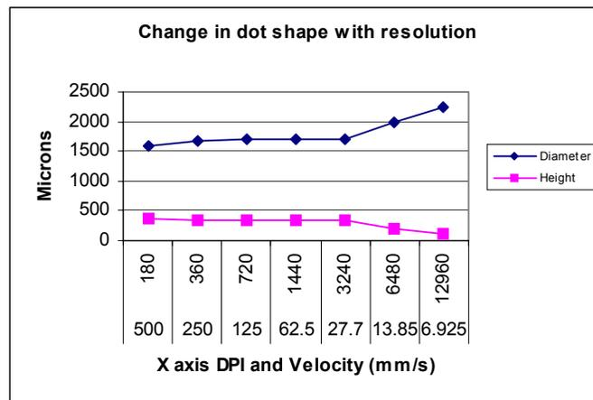
Figure 8: Graph showing affect of print resolution on symbol height and shape.
