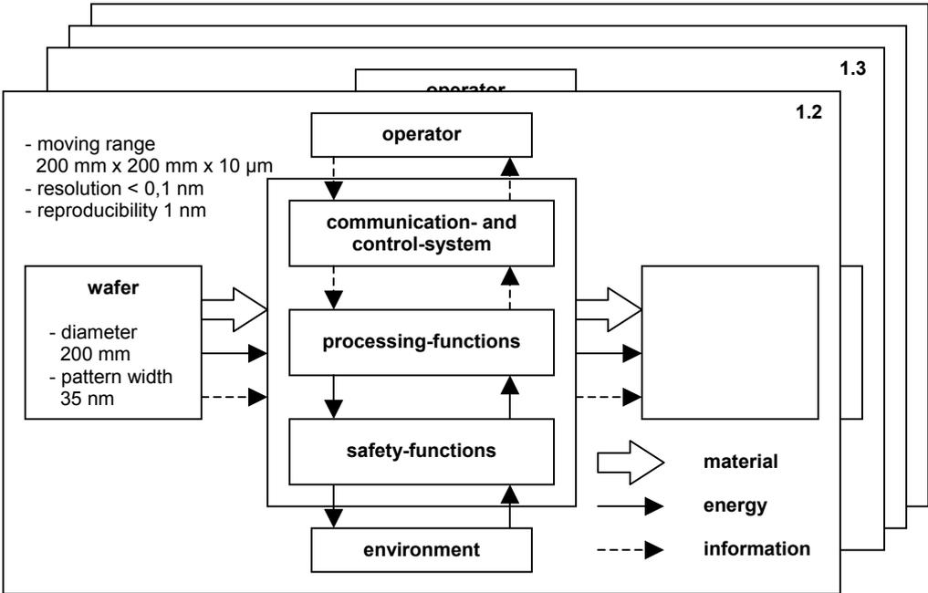
Figure 1. Overall function of a nano-positioning system.
