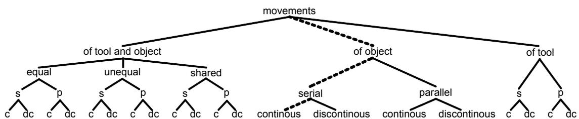
Figure 6. Decision tree for determination of the movements of object and tool (marked path of actual decision).
