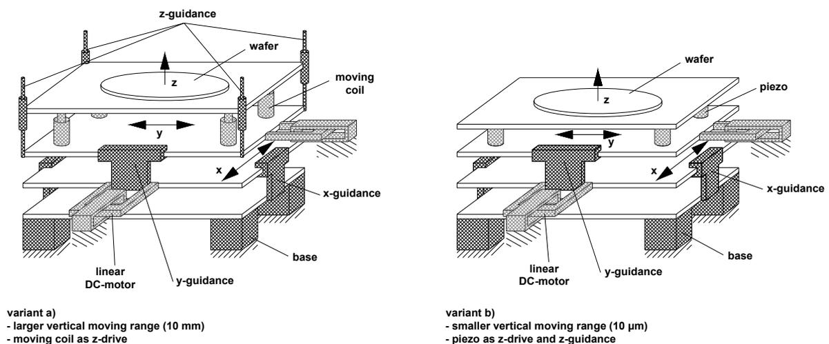
Figure 7. Three coordinate positioning units.
