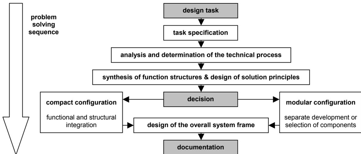
Figure 3. The design process for function-oriented configuration.
