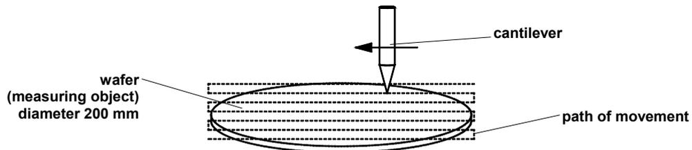
Figure 4. Measuring of an object and the path of relative movement (symbolic).
