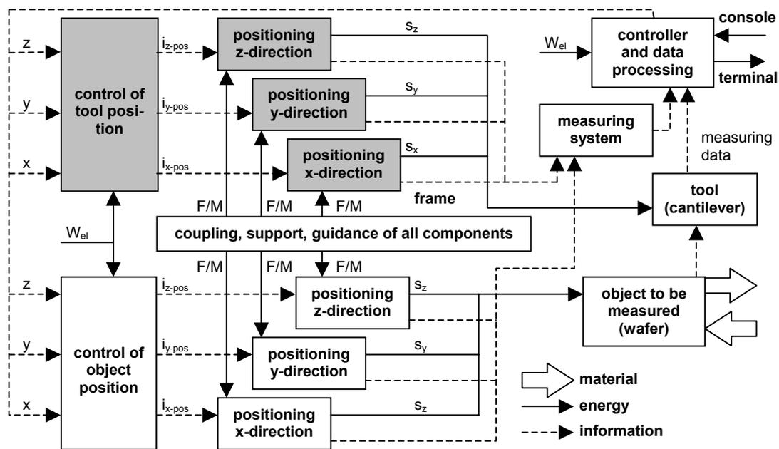
Figure 5. Maximum function structure specified for the wafer inspection by elimination of the shadowed sub-functions.
