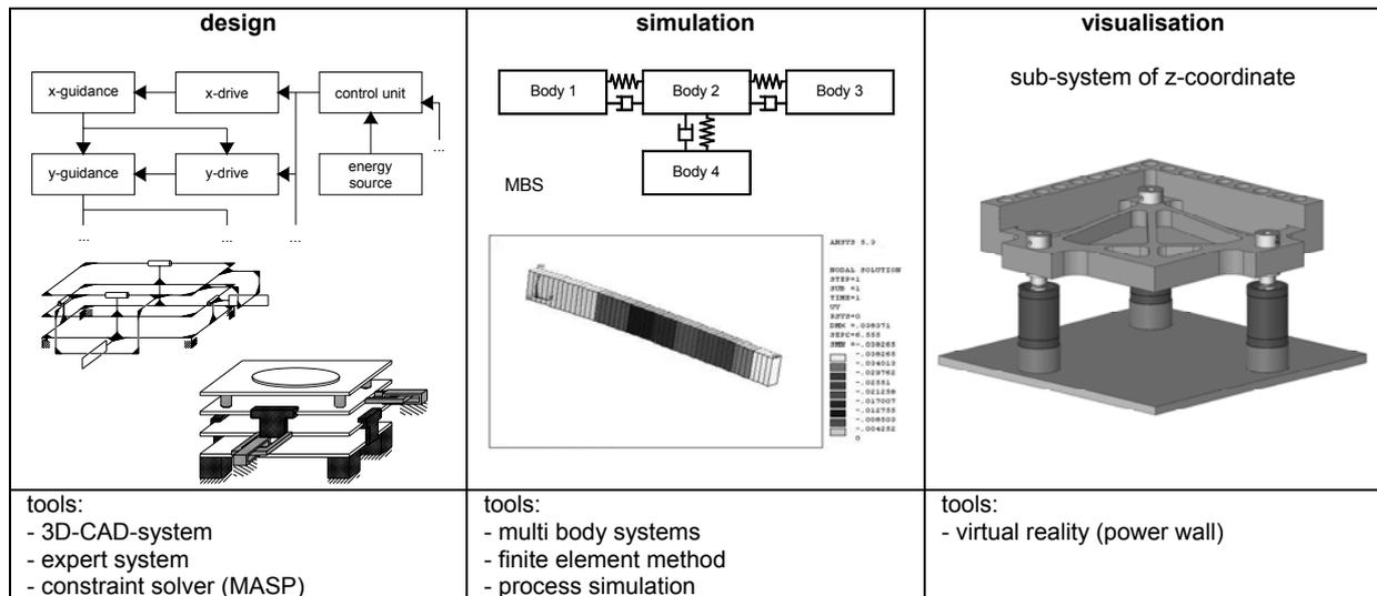
Figure 8. Virtual prototyping in function oriented configuration.
