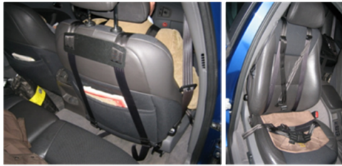
Figure 7. The fixation of the belts in the test Saab 9-5 car
