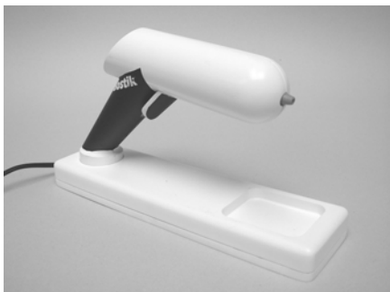
Figure 1: A glue gun model designed to suit manufacture by turning and milling.
