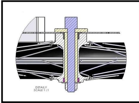
Figure 5 Stub axle
