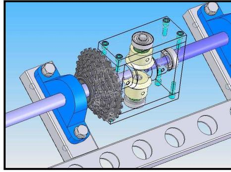
Figure 6 Rear axle assembly
