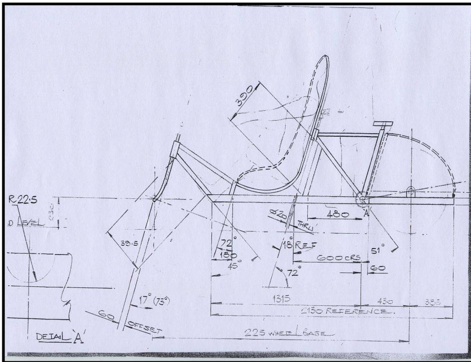
Figure 1 Layout of Tandem with Main Dimensions
