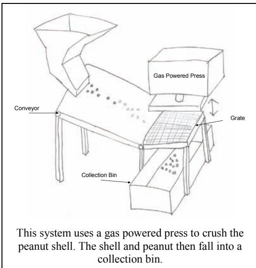
This system uses a gas powered press to crush the peanut shell. The shell and peanut then fall into a collection bin.
