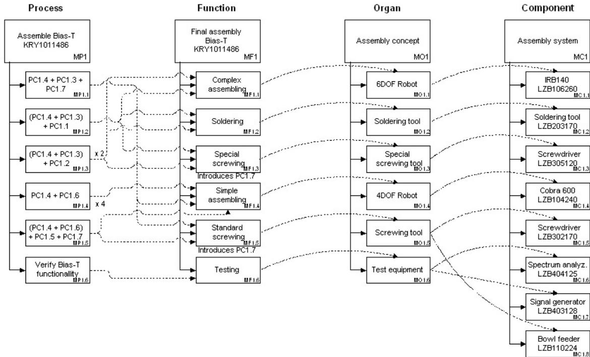
**Figure 4. Decomposition of the Bias-T Manufacturing System**
