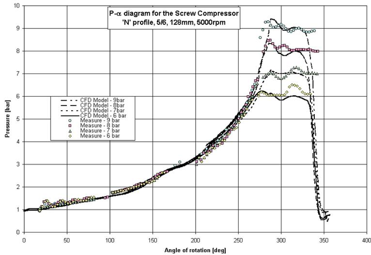
**Figure 3. Pressure-rotation angle diagrams for various discharge pressures**
