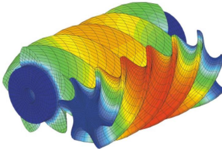
**Figure 4. Rotor deformation**
