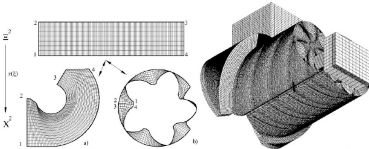
**Figure 2. Left - Patterns of grid topology in a screw compressor
