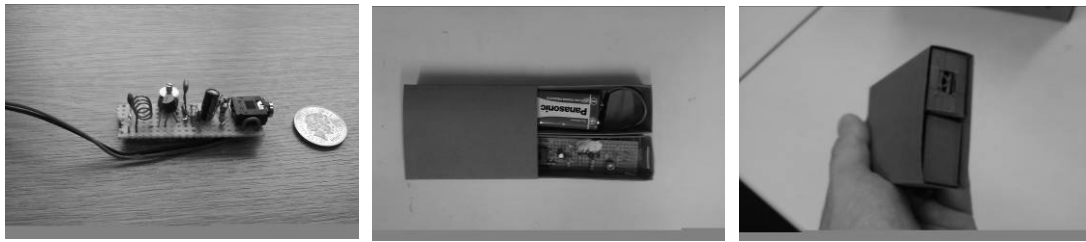
Figure 3. (a) transmitter strip board layout designed by student team; (b) and (c) enclosure for transmitter provides user access to battery and audio plugs.
