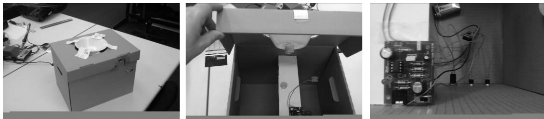
Figure 4. (a) completed product with speaker mounted in box (b) speaker voice coil and magnet configuration (c) amplifier wiring and switch mounting.
