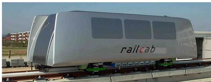
Figure 2. Prototype of the innovative autonomous railway system RailCab (scale 1:2.5)
