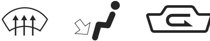
Figure 9. Symbols of air conditioning controls.
