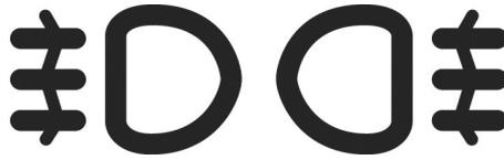
Figure 8. Symbols for front fog lamp (Left) and rear fog lamp (left).
