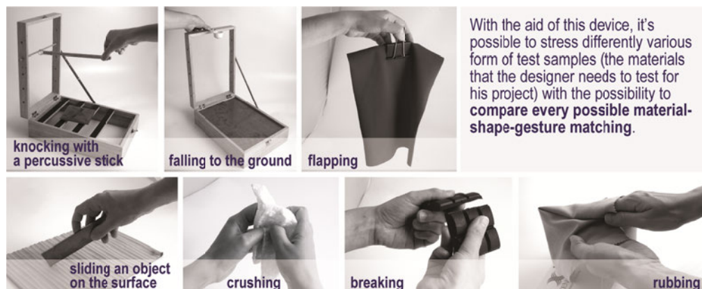
Figure 4. SounBe ® exciting modes: the pictures show seven possible gestures to stress the material samples, giving the possibility to compare every possible material-shape-gesture matching
