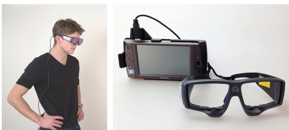
Figure 1. Mobile eye tracking glasses with recording unit
