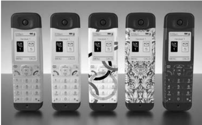
Figure 6. Using heat-shrink material to colour and hold together the DECT phone halves
