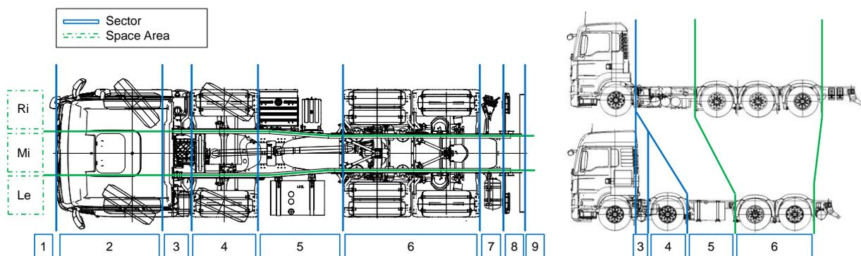
**Figure 2. Generic package space decomposition at MAN. Highlighted sectors 3, 5 and 7 show possible installation space for chassis mounted parts.**
