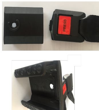
Figure 9: The first sample from Magicfirm Europe, printed in their machine ZYXX+ 3D Printer
